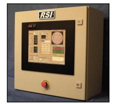
The Model 50 T80XC is a low cost x-ray gauge designed to replace radioisotope "gamma ray" systems, while providing significantly improved thickness measurement...better accuracy, faster response and larger air gaps.
